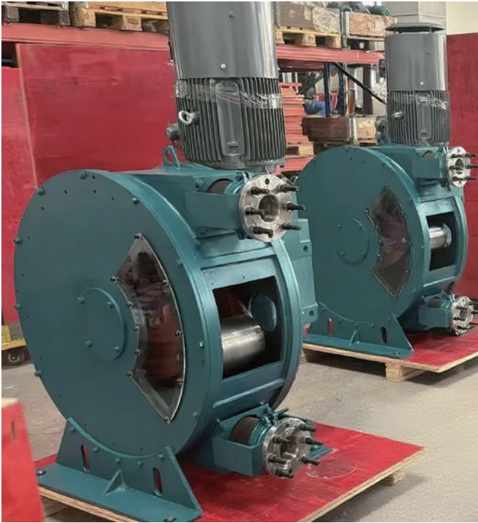
02 ▶ Pumping of high-viscosity materials
